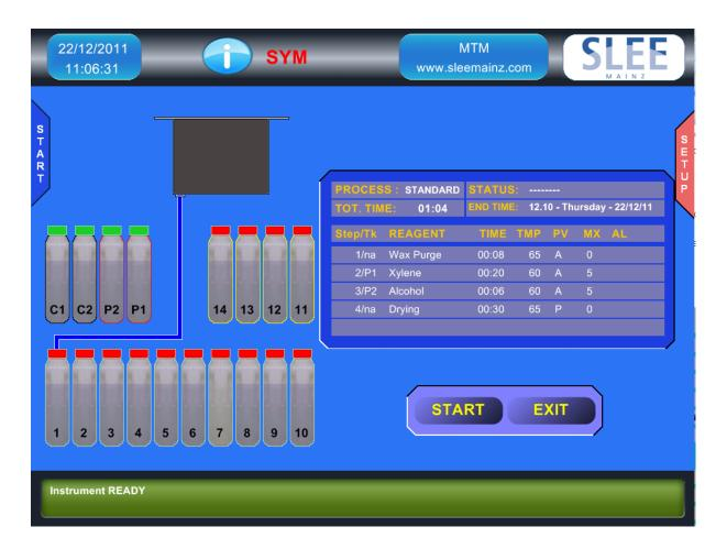
The bottles containing the purge reagents are labelled with P1 and P2 and must contain: (P1) xylene (or substitutes), the second (P2) 95 or 100 % ethanol.
