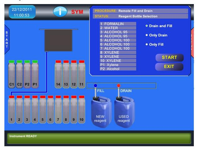
The RFD connectors are placed in the front of the device as shown in the picture. In the left side there is the one for the FILL while in the right there is the one for the DRAIN. To those ports it is necessary to connect the hoses with quick connectors and 90° elbows that will be placed inside the external bottles with the waste and the clean reagent. The RFD can work in three different modalities:
