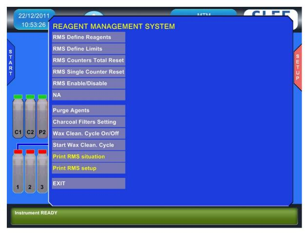
The MTM I RMS is a system to punctually and exactly manage all reagents to guarantee a constant process and sample quality. The use of the Reagent Management System eliminates the need to make annoying written annotations of reagent bottle status. This results in substantial time savings and eliminates the possibility of errors caused by multiple operators using the device.
